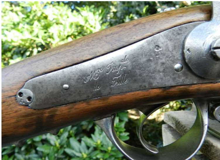
picture 12 Cylinder head screw with holes (French military percussion rifle)
